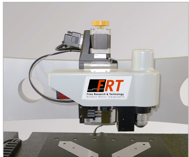
FRT WLI measuring head on MicroProf® 200
